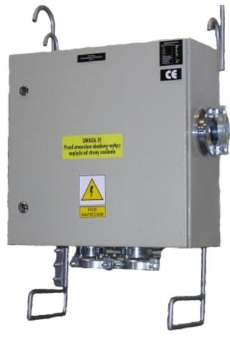
Switchgears type SPR-1 and SPR-2 are an electrical devices designed for use in the underground mining faces in non-explosive hazard conditions and on the ground in environment 2. Switchgears type SPR-1 and SPR-2 are designed for connecting and branching-off mine 3-phase grid circuits with insulated star point of the transformer (IT system) for the grid rated voltage of 500V.
